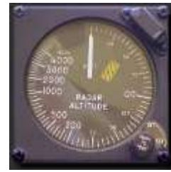
Figure 8: Analogue display of a radar altimeter
