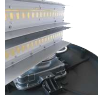
Figure 7: The patch antenna array of a maritime FMCW navigation radar in X-Band
